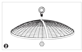
Place Wood Grate into Fire Bowl . Place Cooking Grill into Fire Bowl. Place Fire Screen onto Fire Bowl.
