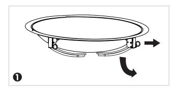
Attach Handle (A) to Fire Screen (B) using Hex Nut (f).
